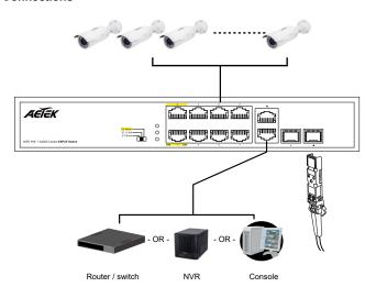
Use SFP, LC type transceiver with 100Mbps or 1Gbps transfer speed in Single mode (10km,30km,50km,80km) or Multi mode (0.5m or 2km) or Bidi (10km,30km,50km,80km).
